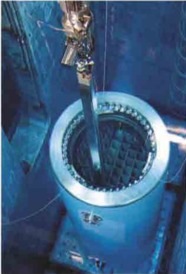
Spent fuel is transferred to the interim storage facility in a transfer tank made of spheroidal graphite cast iron. Its walls are 36 centimetres thick, and it weighs 93 tonnes when fully loaded.
